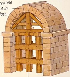
The frame was removed once the arch was completed.
